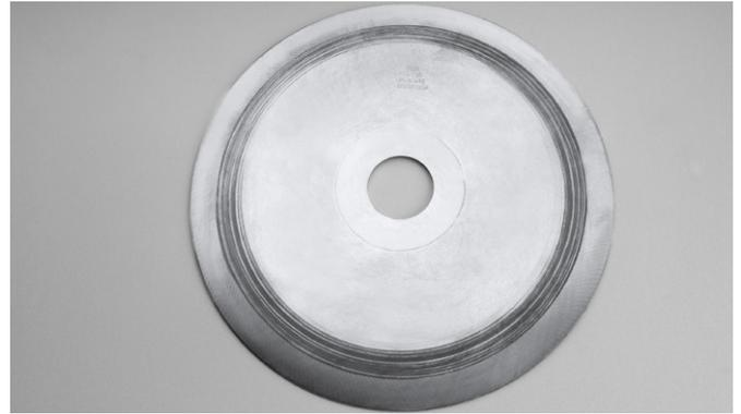
**2** Cut the hose by using a sharpened cutting disc - do not use an abrasive disc. Avoid causing damage to the wire braid during cutting. Clean the hose carefully from cutting residue.
