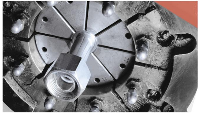
**8** Ensure that the full length of the ferrule is covered by the dies
