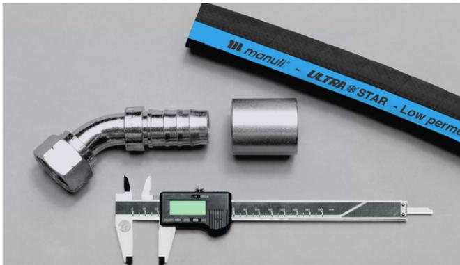
**1** Check the dimensions of the components
