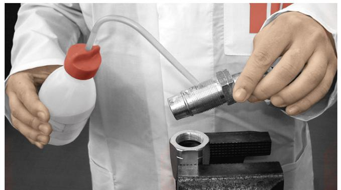
**6** Secure the hose and socket vertically in the bench-vice. Using a suitable oil, generously lubricate the thread and taper of the fitting as well as the inside of the hose and socket.
