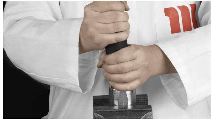
**4** Secure the socket vertically in a bench-vice and screw in the hose, turning counter-clockwise, until it reaches the bottom of the socket. Unscrew the hose by  $\frac{1}{4}$  turn to prevent damage in later steps.
