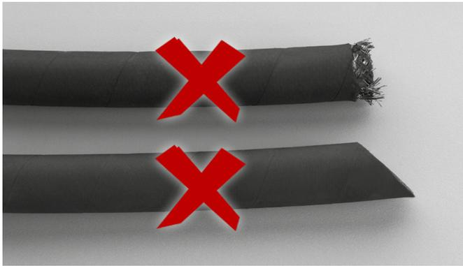
**3** The end of the hose should be cut squarely to  $\pm 2^\circ$  and there should be no ragged edges
