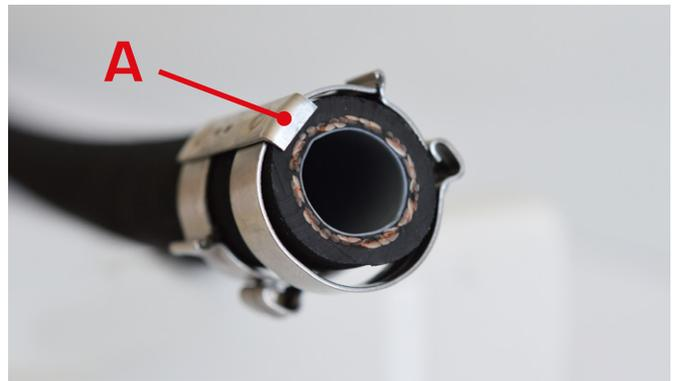
**4** Place the double clamp on the hose so that the tooth on the bar (A) comes into contact with the end of the hose that has been cut
