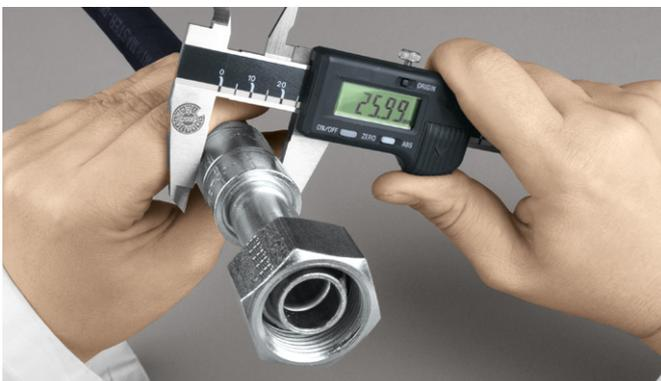
**10** Inspect the crimped dimension using a calibrated vernier. Check the diameter at the centre of the ferrule against the relevant value in the latest version of the crimping data
