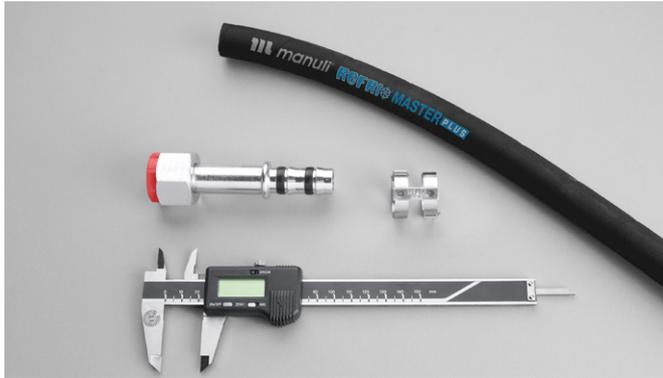
**1** Check the dimensions of the components
