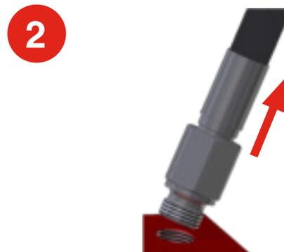
Remove the adaptor and insert as a single piece.
