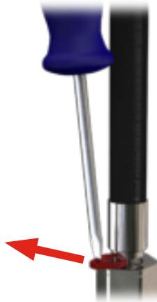
Use a flat-headed screwdriver, or similar tool, to remove the safety clip.
