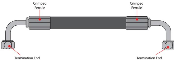
Fig. 3 - Complete hydraulic hose assembly
