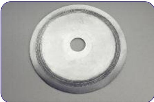
**4** Cut the hose by using a proper sharpened disc (see fig. 4), **do not use an abrasive disc**. The hose must be square and clean cut. Avoid cutting the hose not perpendicularly or cutting the hose causing damages on its wire braid (see fig. 2, 3) for a proper cutting hose operation. Clean the hose carefully from any cutting residue.
