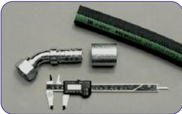
**1** Check the dimensions of the components.
