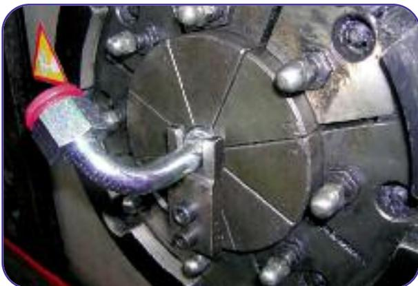
**7** Set up the crimping machine selecting the die set that is closed to the dimension specified diameter. Place the fitting on the proper positioner to ensure that it is in the correct position (table c).
