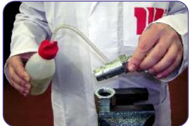
**7** Position the hose complete with socket i.e. by using a bench vise. Grease with a lot of oil the threading and the taper of the fitting as well as the inside of hose.
