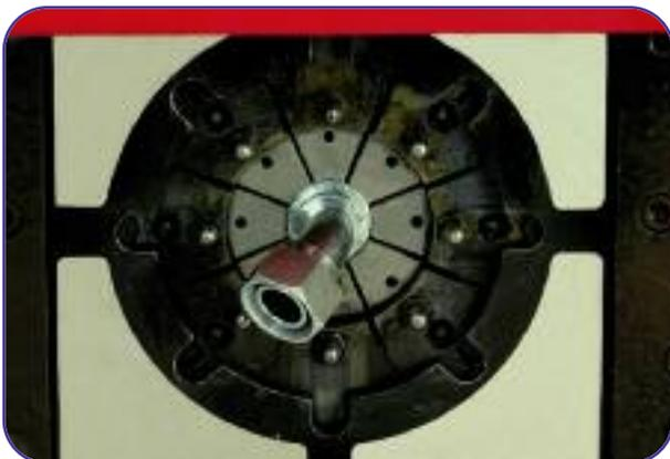
**8** Set up the crimping machine selecting the die set that is closed to the specified dimension. Crimp to the specified diameter. Ensure the dies fully cover the ferrule length.
