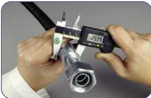
**9** Inspect the crimping dimension using a calibrated vernier. Check the diameter at the centre of the ferrule following the values in table a.
