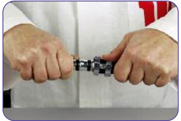
**6** Find the correct orientation and insert completely the fitting into the hose.
