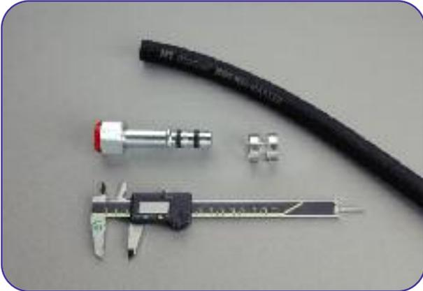
**1** Check the dimensions of the components.
