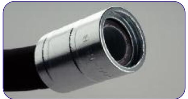
**4** Place the ferrule on the flexible hose so that the ferrule tooth touches the end of the cut hose.
