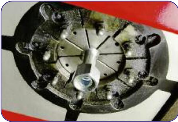
**7** Set up the crimping machine selecting the die set that is closed to the specified dimension. Crimp to the specified diameter (table a). Ensure the dies fully cover the ferrule length.
