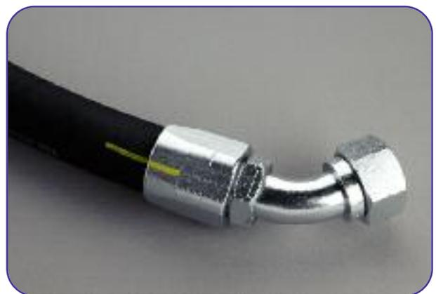
**9** You can leave a margin of max 3 mm between the hexagon of the fitting and the socket. Verify alignment.
