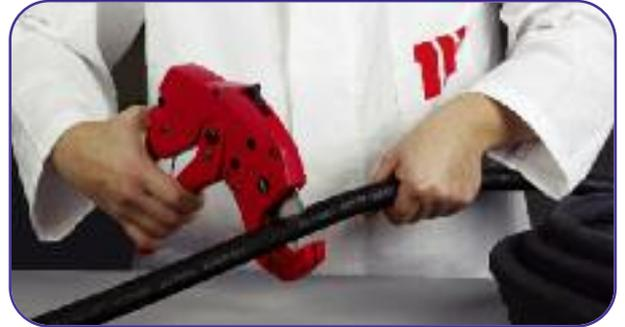
**2** Cut the end of the hose in a perpendicular direction, using the manual cutter.
