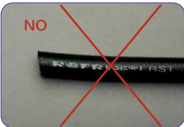
**3** Verify the end of the hose to be cut in a perpendicular direction.
