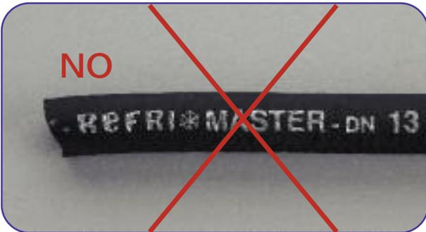
**3** Verify the end of the hose to be cut in a perpendicular direction.
