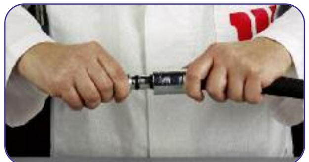
**6** Find the correct orientation and insert completely the fitting into the hose.
