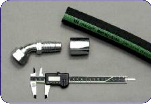
**1** Check the dimensions of the components.
