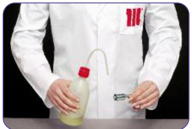
**4** Grease the end of the fitting joint with the same oil used in the air conditioning system.
