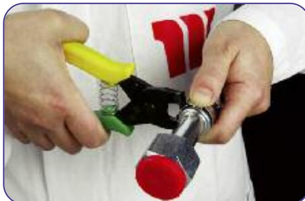
**9** Tighting the double clamp until click to close. Reverse the position of the pliers to open.
