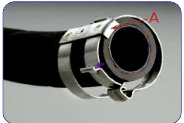
**4** Place the double clamp on the flexible hose in such a way that the tooth of bar A comes contact with the end of the hose that has been cut.
