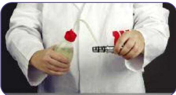
**5** Grease the end of the fitting joint with the same oil used in the air conditioning system.
