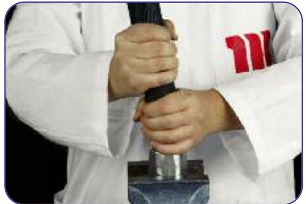
**5** Secure in position the socket i.e. by using a benchvise. Screw the hose counterclockwise into the socket until it reaches the bottom. Unscrew 1/4 turn to prevent damage in screwing.
