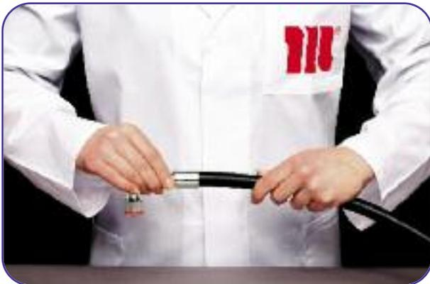
**5** Find the correct orientation and insert completely the fitting into the hose.
