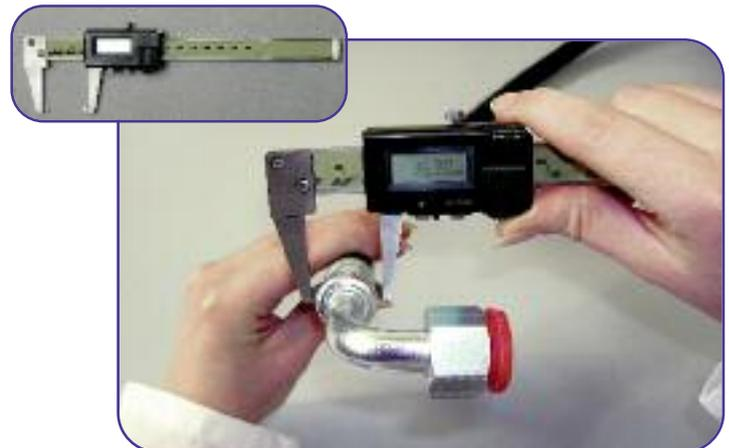
**8** Inspect the crimping dimension using the proper calibrated vernier. Check the dimensions following the values in table c.
