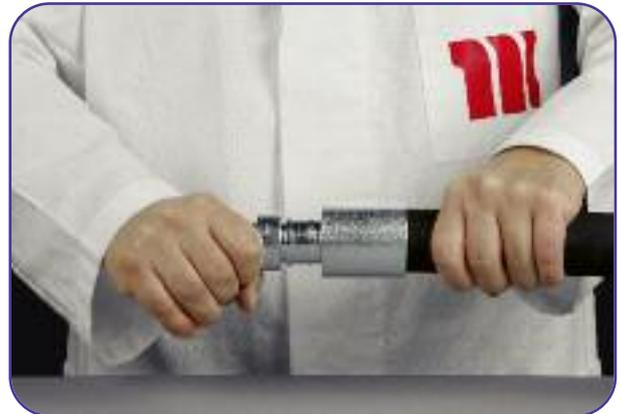
**7** Find the correct orientation and insert completely the fitting into the hose.
