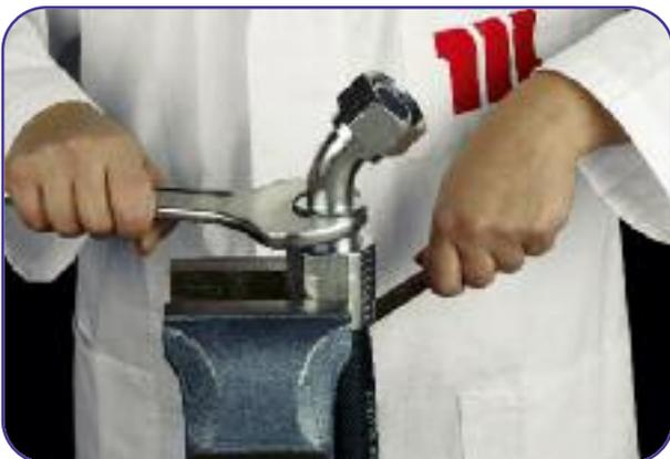
**8** Insert the fitting into the hose. Press slightly and screw by hand turning clockwise the first threads. Then by using an appropriate spanner or a screwspanner on the hexagon, screw the fitting into the socket with a continuous and constant rotation motion and verify any absence of hose rotation inside the socket during the fitting screwing. Complete the screwing until the fitting reaches the bottom against the socket. Never overtighten. Assembling is now finished.
