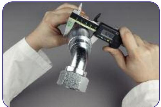
**9** Inspect the crimping dimension using a calibrated vernier. Check the diameter at the centre of the ferrule following the values on the table b.
