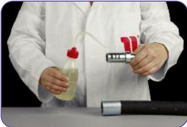
**6** Grease the end of the fitting joint with the same oil used in the air conditioning system.
