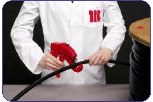
**2** Cut the end of the hose in a perpendicular direction, using the manual cutter.
