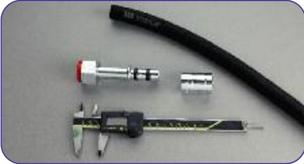
**1** Check the dimensions of the components.
