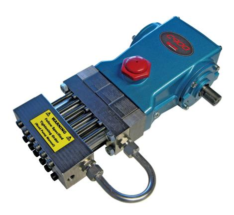
C900 pump is a triplex type positive displacement high pressure pump with spring operated suction and pressure valves. C900 pump consists of oil lubricated drive end and fluid end in contact with the pumped media. The body of the drive end is of casted alloy. Parts that come in contact with pumped media are of stainless steel (1.4401, AISI 316, or better from the corrosion point of view), special plastics and construction ceramics (Al2O3).
