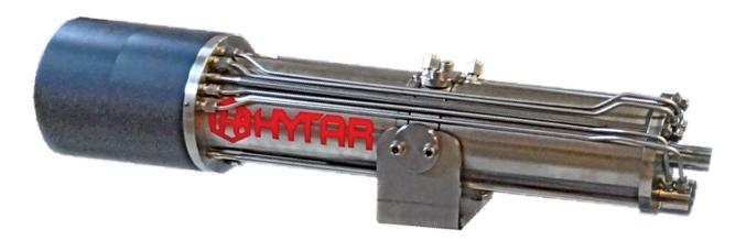
PSPO-8 is a pneumatically operated shower pipe oscillator for demanding applications with slow speed oscillation. Smooth movement at slow speed is ensured by hydraulic brake (hydraulic oil, glycol or water brake available). Oscillation speed can be adjusted either by pneumatic pressure regulator or I/P transducer or by adjusting the brake.
