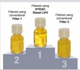
The evidence is a comparison between three diesel samples after filtration and dewatering. The particular purity of the diesel dewatered and filtered with HYDAC LowViscosity Housings (LVH) is already evident with the naked eye.
