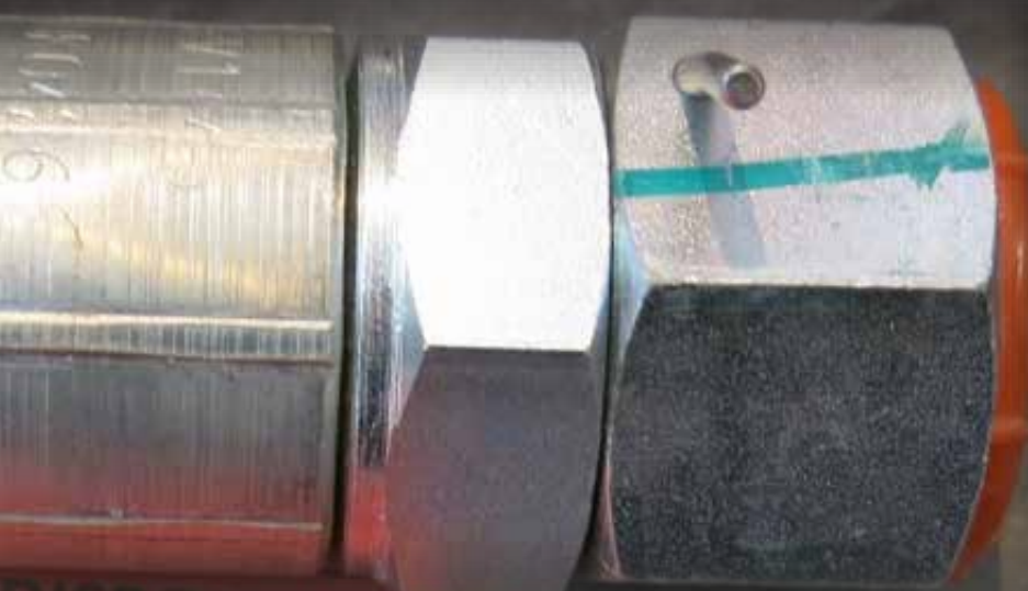
Thrust-wire protruding from termination end
