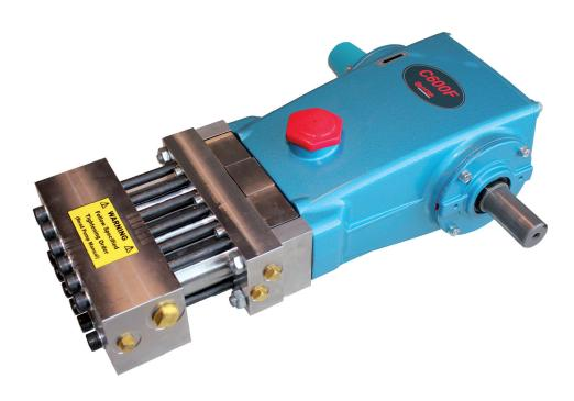
C600F pump is a triplex type positive displacement high pressure pump with spring operated suction and pressure valves. C600F pump consists of oil lubricated drive end and fluid end in contact with the pumped media. The body of the drive end is of casted alloy. Parts that come in contact with pumped media are of stainless steel (1.4401, AISI 316, or better from the corrosion point of view), special plastics and construction ceramics (AI2O3).
