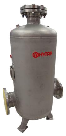
HY100 suction stabilizer is installed in the suction line of plunger pumps in flow through configuration. Suction stabilizer isolates the pump from the suction piping and offers dampening of flow and acceleration pulsations. Suction stabilizer eliminates the pressure loss created by pulsating flow and increases system's NPSHa value. Hytar HY100 suction stabilizer can be equipped with a bleeding valve allowing air removal from the fluid.
